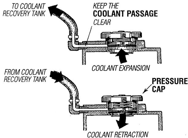
**NOTE:** Periodically check the condition of the manifold pressure cap. Ensure the upper and lower rubber seals are in good condition. Check to ensure the vacuum valve opens and closes tightly. Carry a spare cap. Check also to ensure the coolant passage is clear so coolant within the system is able to expand and contract to and from the coolant recovery tank.
