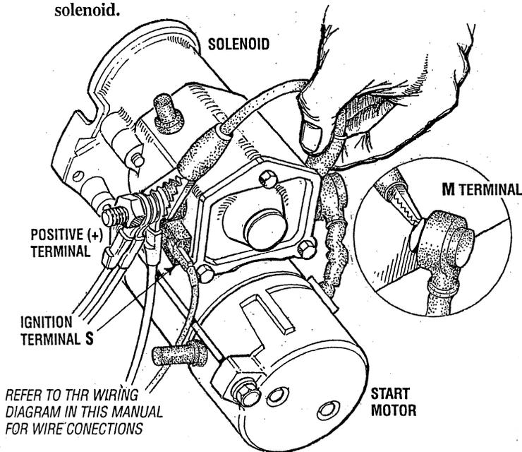
**NOTE:** *Starter motors are either inertia type or pre-engaged. In the pre-engaged model, the solenoid also moves an arm that engages the starter motor to the flywheel of the engine. using a screwdriver to bypass the solenoid on such a starter will run the motor without engaging the flywheel.*
