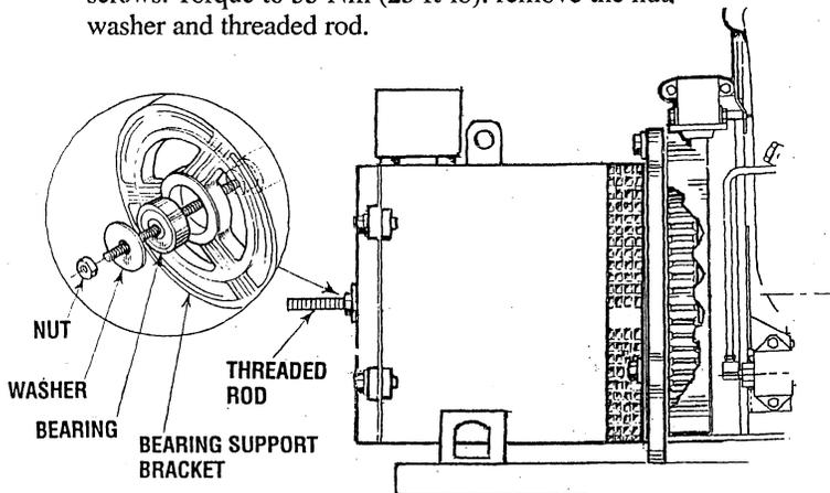
4. Rotate the generator by hand two full revolutions to ensure the generator rotates freely. Reinstall the rear vent cover.
