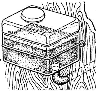
INSPECT AND CLEAN THE COOLANT RECOVERY TANK AND ITS CONNECTING HOSE EVERY 3 MONTHS
