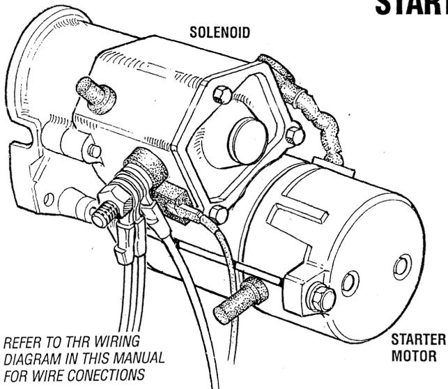
The starting system includes the battery, starter motor and solenoid, and the ignition switches - Start/Preheat.
