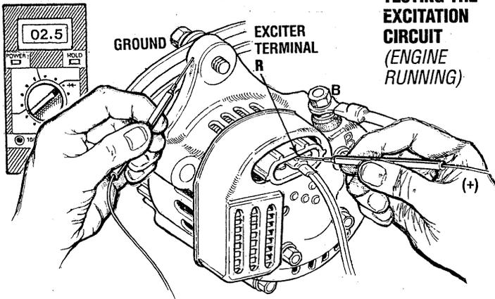
3. If the reading is between .75 and 1.1 volts, the rotor field circuit probably is shorted or grounded.
