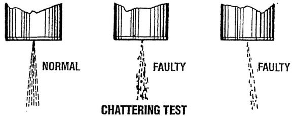
2. Apply the pressure of 1635 lb/in<sup>2</sup> (115 kg/cm<sup>2</sup>) to nozzle by operating the hand lever, and check the drips from the nozzle tip. If it drips or has a large accumulation of fuel on the bottom, it is considered defective and should be replaced. A very small amount of fuel may sometimes remain on the tip of the nozzle; however, this does not indicate a defect.
