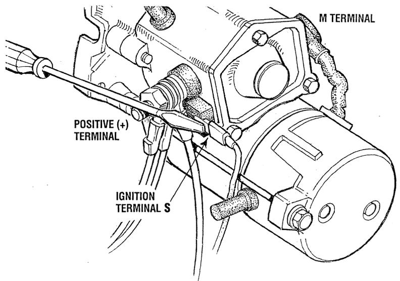
**If nothing happens at all, the solenoid is not getting current..** Check the battery and inspect the wiring connections. It is also possible that the solenoid is defective.
