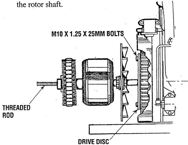
2. With the aid of a sling or fabricated lifting eye, support the stator housing assembly and carefully guide it over the rotor assembly until the rear bearing contacts the bearing boss in the rear support.
